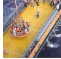
Photograph 2: Conventional baskets require the riders to perch on the outer ring.
