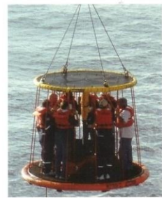
Photograph 3: The world's first 12-man X-904 personnel basket—a safer design than a conventional flexible basket.
