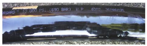
Figure. Photograph of hose cover after the N2 pressure test
